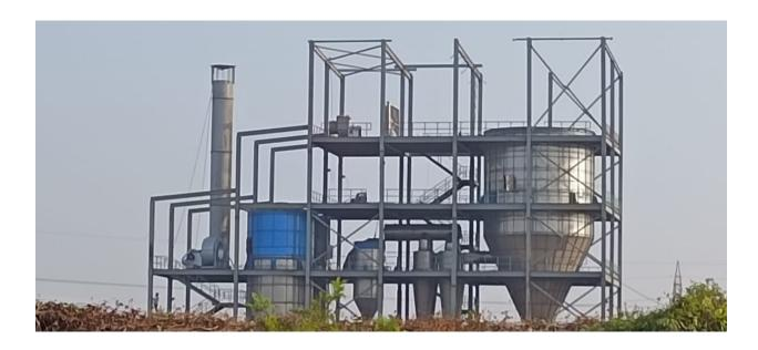
A <u>spray dryer</u> is a device that transforms a liquid feed into a dry powder in a single continuous step. This is achieved by atomizing the liquid into a fine spray of droplets and then rapidly drying these droplets in a hot gas stream. The basic working principle involves the following stages:
